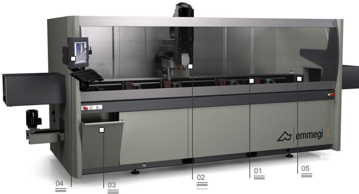
CNC machining centre, with 3 controlled axes; the spindle has an automatic tool slewing system on 3 fixed positions that allows processing on 3 sides of the workpiece.
