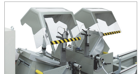
Tilting of the moving cutting heads 02
